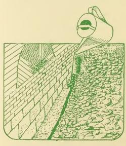
trench 6 to 8 inches wide and a few inches deepnext to the walls or piers, taking care not to go below the top of the footing. If the land slopes or the footing is more than 12 inches deep, make crowbar, pipe, or rod holes about an inch in diameter and a foot apart, from the bottom of the trench to near the footing. This will help to distribute the chemical evenly along the wall.
